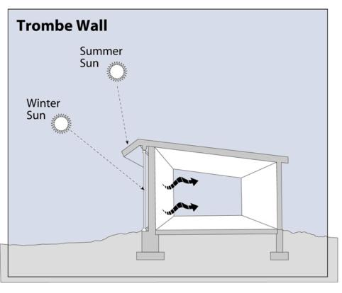
or less in front of the dark-colored wall absorbs solar heat, which is stored in the wall's mass. The heat migrates through the wall and radiates into the living space.
